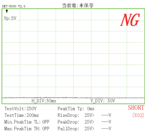
【E02】短路: 隔离膜破损或电芯内部有金属异物导致的短路。 【E02】 SHORT: caused by damaged isolation film or metal particles inside the battery cell.
